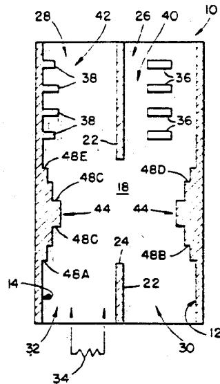
**Cavity Resonator Coupling-Type Power Distributor/Power Combiner Comprising Coupled Input and Output Cavity Resonators**
